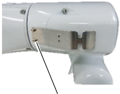
Hexagon socket head cap bolt 2-M4×10
