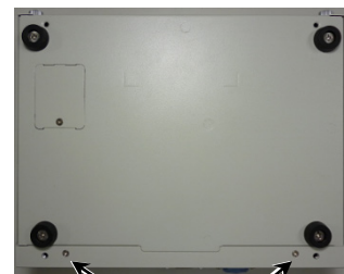
Screws fixing the front cover (Top face) Screws fixing the front cover (Bottom face)
