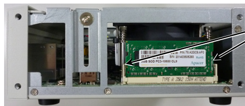
Clips on the sides of the memory socket
