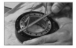
(5) Set the O-ring removed in the removal step (6) into the O-ring (between the Arm #1 and the reduction gear unit) groove of the Arm #1 and install the flexspline on the Arm #1.
