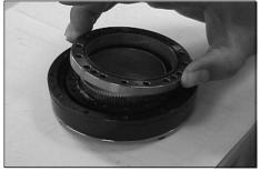
(4) Match the screw holes on the inner ring of the cross roller bearing unit and the through holes of the circular spline.
