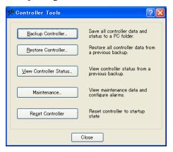
(2) To check the controller Maintenance information, click the <Maintenance> button and display the [Maintenance] dialog box.
