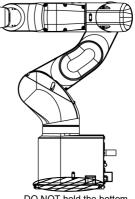
DO NOT hold the bottom of the base by hand.
