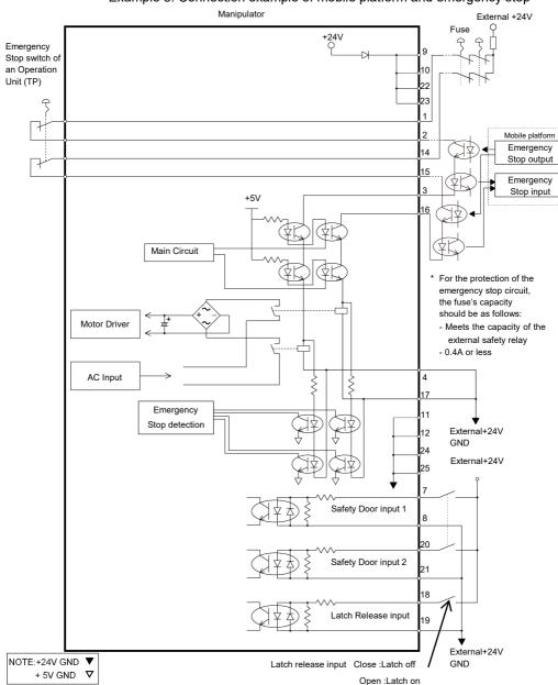
Example 3: Connection example of mobile platform and emergency stop
