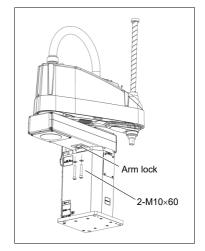
(4) Remove the bolts securing the wire ties removed in step (2).
