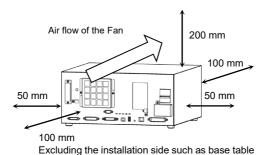
Air with higher temperature than the ambient air (about 10 deg C) is blown out from the exhaust port of the Controller.
