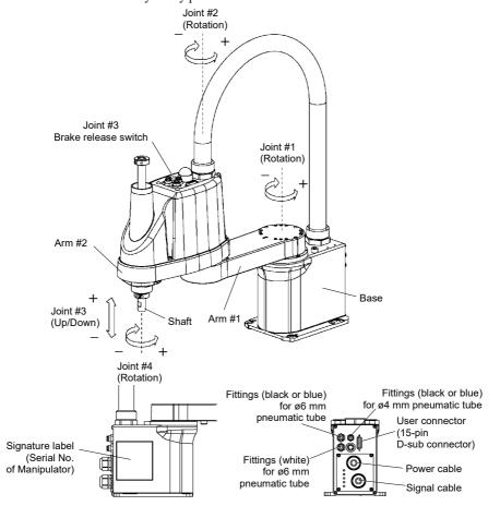
When the system is placed in emergency mode, push the arm or joint of the Manipulator by hand as shown below:
