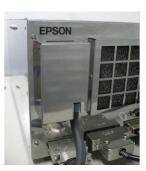
(4) Secure the cover with the screw.
