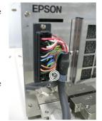
(2) Set the M/C Power Cable in the clamp for the M/C Power Cable.
