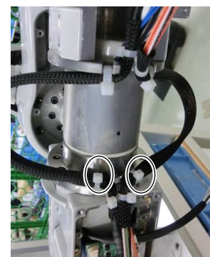
Wire Tie for Prevent Disconnection of Braided Tube
