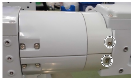
Cross recessed binding head machine screw: 2-M3×6 (×2)
