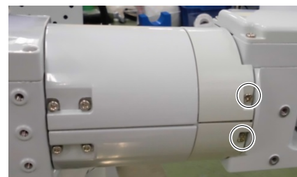
Cross recessed binding head machine screw: 2-M3×6 (×2)
