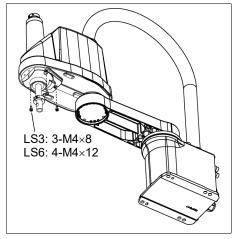
When bellows are installed to the manipulator, remove or pull down the lower bellows and then remove the arm bottom cover. For bellows removal, refer to Maintenance 9. Bellows.
