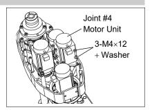
(2) Remove the Joint #4 intermediate shaft unit.
