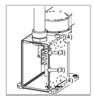
(4) Remove the screws (flat head screw ×4) on the side face of the Base.
