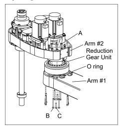
Joint #2 Reduction Gear Unit Installation
