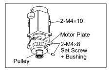
Joint #4 motor Installation
