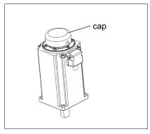
(3) Loosely secure the Joint #3 motor unit to Arm #2.
