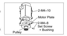
Tighten one of the set screws vertically on the flat face of the motor shaft.
