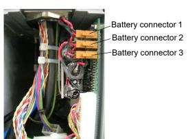
(8) Disconnect the Battery connector 2 and Battery connecter 3, then connect new ones.
