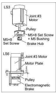
Tighten one of the set screws vertically on the flat face of the motor shaft. Insert a bushing into the other set screw hole to prevent damage to the motor shaft.
