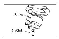
(2) Mount the pulley and brake hub to the Joint #3 motor.
