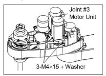
(10) Remove the Joint #3 motor from the Joint #3 motor unit.
