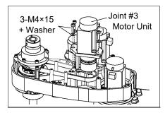
(11) Remove the screws for the spline plate.
