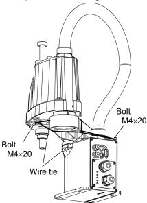
(3) Hold the bottom of Arm #1 by hand to unscrew the anchor bolts. Then, remove the Manipulator from the base table.
