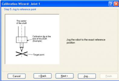
(16) Execute the procedure in "Calibration Using Right / Left Arm Orientations" to accurately calibrate Joint #2.
