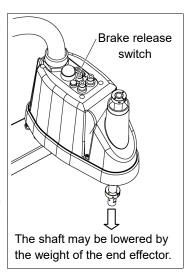
This button switch is a momentary-type; the brake is released only while the button switch is being pressed.
