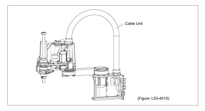
■ If the connectors have been disconnected during the replacement of the cable unit, be sure to reconnect the connectors to their proper positions. Refer to the block diagrams.
