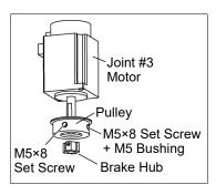
Joint #3 brake Installation (1) Mount the brake to the brake plate.
