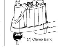
(9) Wipe off the old grease from the lower part of the shaft, and then apply new grease.
