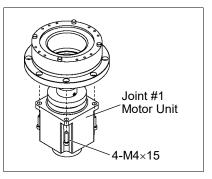
LS6: Loosen the motor flange mounting screws on the Joint #1 motor flange and remove the motor unit
