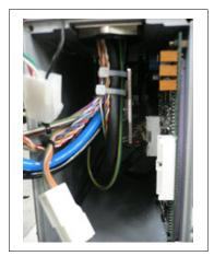
(4) Connect the three batteries connectors and M/C signal connector.
