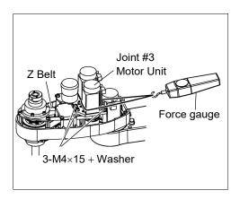
NOTE To check belt tension with the tension meter, refer to Maintenance: 7.4 Checking the Timing Belt Tension (Z Belt).
