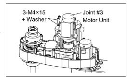
(12) Loosely secure the Joint #3 motor unit to Arm #2.
