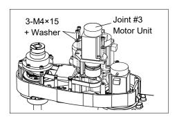
(6) Remove the Joint #3 motor from the Joint #3 motor unit.
