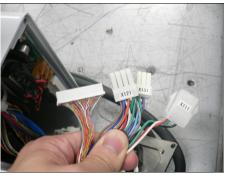
(5) Remove the Connector Sub Plate.
