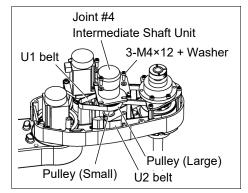
(2) Loosely secure the Joint #4 intermediate shaft unit.
