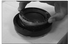
(4) Match the screw holes on the inner ring of the cross roller bearing unit and the through holes of the circular spline.
