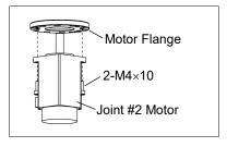
Joint #2 Motor Installation
