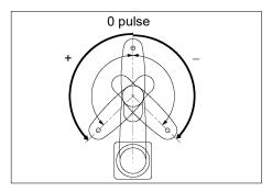
0 pulse position of Joint #3: upper limit position in motion range
