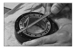
(5) Set the O-ring removed in the removal step (6) into the O-ring groove of the Arm #1 and install the flexspline on the Arm #1.
