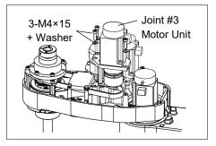
(11) Remove the screws securing the Joint #4 motor unit and pull out the motor unit.
