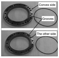
(3) Face the convex side of the circular spline down, and then fit it into the flexspline.
