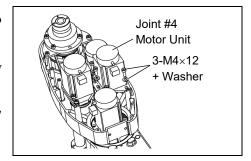
(5) Apply the proper tension to the U1 belt, and then secure the Joint #4 intermediate shaft unit.
