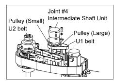
(5) Loosely secure the Joint #4 intermediate shaft unit.
