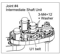
U1 belt Installation (1) Keeping the U1 belt on the large pulley of the Joint #4 intermediate shaft unit, set the U2 belt in the Arm #2 on the small pulley and put them on the Arm #2 upper surface.
