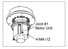
(7) Remove the waveform generator from the Joint #1 motor.
