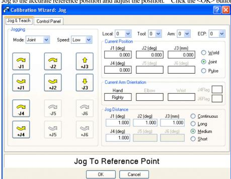
Jog to the accurate reference position and adjust the position. Click the <OK> button.
