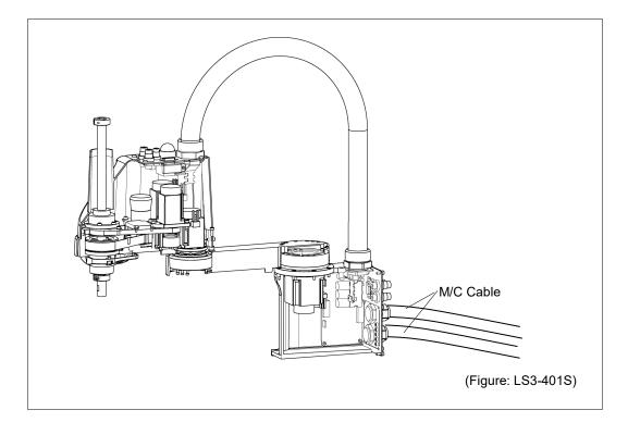
If the connectors have been disconnected during the replacement of the cable unit, be sure to reconnect the connectors to their proper positions. Refer to the block diagrams.
