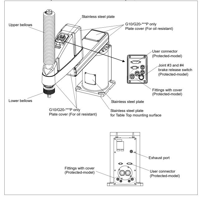
NOTE For Protected-model, all the screws used for outer parts are stainless steel screws. (Excluding the screw used for mechanical stop.)
