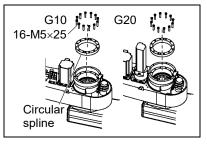
Joint #2 reduction gear unit Installation
