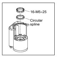
Joint #1 reduction gear unit Installation (1) A new reduction gear unit contains the parts shown in the picture on the right when it is unpacked.
