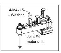
(14) Apply the proper tension to the Z belt and U belt, and then secure the Joint #3 motor unit and Joint #4 motor unit.
