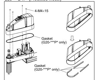
Gaskets are installed to G20-\*\*\*P\*.
