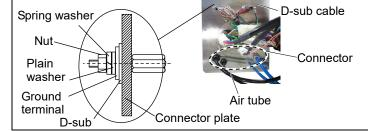
(8) Loosely mount the connector plate with 2 screws (M4).
