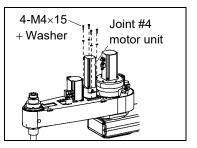
(8) Apply the proper tension to the Z belt and U belt, and then secure the Joint #3 motor unit and Joint #4 motor unit.
