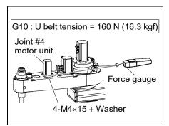
NOTE Loosely secure the Joint #4 motor unit to Arm #2 so that the motor unit can be moved by hand, and it will not tilt when pulled. If the unit is secured too loose or too tight, the belt will not have the proper tension.
