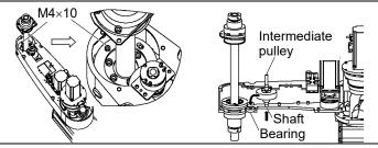
(4) Remove the bolt of the Z gear.
