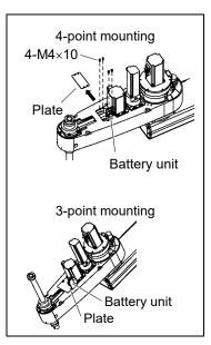
When you use the plate of 3-point mounting, loosen the plate mounting bolts.
