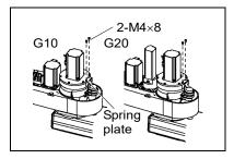
(9) Remove the Joint #2 motor unit from Arm #2.
