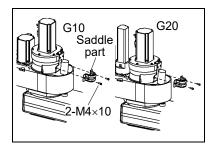
(14) Connect the connectors and the ground wire.
