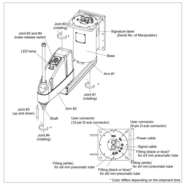
NOTE - The brake release switch affects both Joints #3 and #4. When the brake release switch is pressed in emergency mode, the brakes for both Joints #3 and #4 are released simultaneously.
