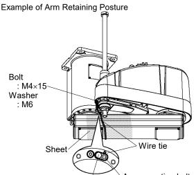
Bolt for Arm #1 mechanical stop Arm mounting bolt
