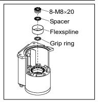
(5) Remove the circular spline from the base.
