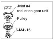
Joint #4 (1) Mount the U pulley. Reduction gear unit Installation: G20
