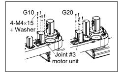
(5) Apply the proper tension to the Z belt, and then secure the Joint #3 motor unit.
