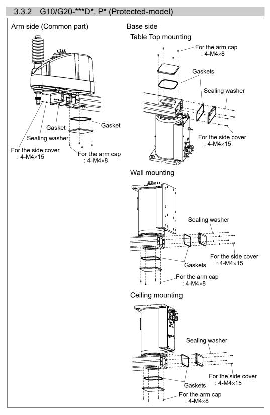
Gaskets and sealing washers are installed to G10/G20-\*\*\*D\*, P\* (Protected-model).
