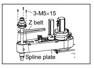
Z belt(1)Pass a new Z belt through the shaft from above, and then place it under the splineInstallation : G20plate.
