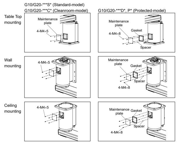
A gasket and spacers are installed to G10/G20-\*\*\*D\*, P\* (Protected-model).
