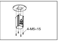
Joint #2 motor (1) Mount the motor flange on the Joint #2 motor.
