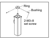
Joint #4 motor Removal: G20 (1) Mount the ring to the Joint #4 motor.
