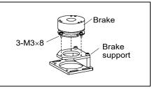
(3) Mount back the Joint #3 brake unit to Arm #2.
