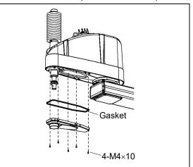
A gasket is installed to G10/G20-\*\*\*C\* (Cleanroom-model) and G10/G20-\*\*\*D\*/P\* (Protected-model).
