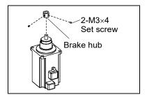
Joint #3 brake (1) Mount the brake hub to the Z1 pulley. Installation
