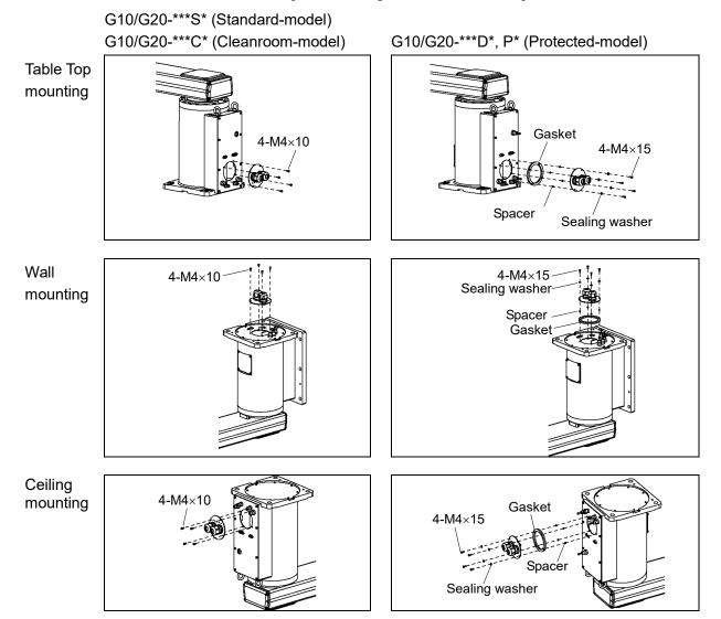
A gasket, spacers, and sealing washers are installed to G10/G20-\*\*\*D\*, P\* (Protected - model).
