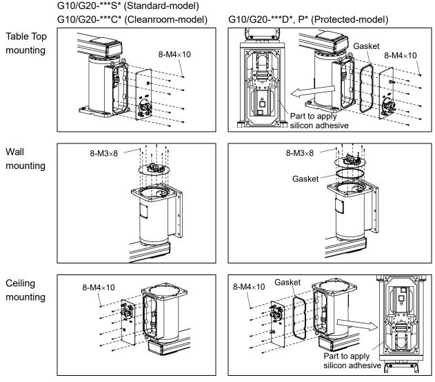
A gasket is installed to G10/G20-\*\*\*D\*, P\* (Protected-model).
