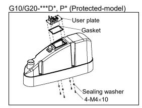
A gasket and sealing washers are installed to G10/G20-\*\*\*D\*, P\* (Protected-model).
