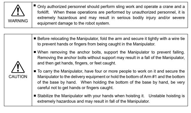
When transporting the Manipulator for a long distance, secure it to the delivery equipment so that the Manipulator cannot fall.
