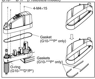
Gaskets are installed to G10-\*\*\*P\*. O-ring is installed to G10-\*\*\*D\*, P\*.
