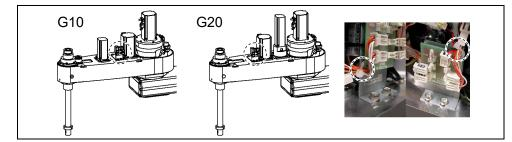
(5) Disconnect the connectors X61, X62, X63, and X64 connected to the battery board.
