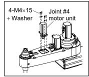
(9) Remove the U1 pulley and the motor plate from the Joint #4 motor.
