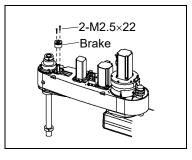
Joint #4 brake (1) Mount the brake. Installation: G10
