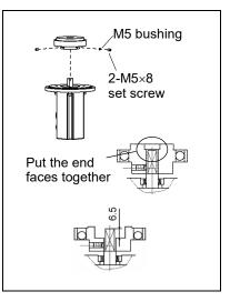
(3) Mount the waveform generator on the Joint #2 motor.
