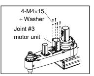
(10) Remove the Joint #4 motor unit from Arm #2.
