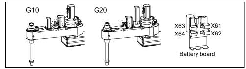
(6) Loosen the screws securing the battery board and remove the battery board.
