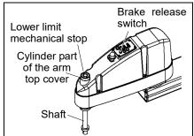
When bellows are installed to the manipulator, install the arm top cover and then install the upper bellows. For bellows installation, refer to *Maintenance 9. Bellows*.
