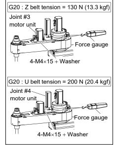
(9) When you use the plate of 4-point mounting, mount the plate without pressing it to the motor.
