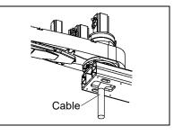
(10) Mount the spring for cable protection to the spring plate with a wire tie.
