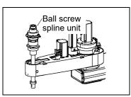
(1) Pass the Z belt through the shaft and mount the ball screw spline unit to Arm #2.
