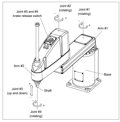
Move the shaft while pressing the brake release switch.
