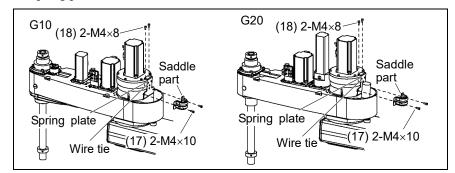
(17) Cut off the two wire tie binding cables.
