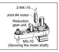
(8) Remove the ring from the Joint #4 motor.
