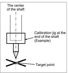
After removing the end effector and performing the calibration, install the end effector and move the Manipulator to the teaching point to verify whether there is a positional gap. If there is a positional gap, fine-tune the installation position of the end effector and teach the point again.
