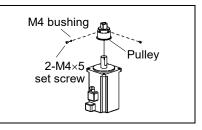
Joint #3 motor (1) Secure the pulley to the new motor shaft.
