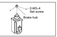
(2) Mount the brake support to the brake.
