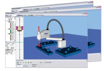
The Epson RC+ Simulator allows you to carry out risk-free testing, comparison and process visualisation before any robot implementation.
